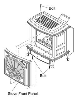
Figure 51 - Removing Front Panel from Stove
